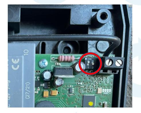
To alter the dip switches this must be done within 30 seconds of powering on the control panel
