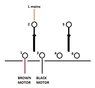
The BLACK and BROWN wires coming from the motor are directional wires, so may need to be swapped over if the operational direction is incorrect. (i.e up button taking the door down & vice versa)
