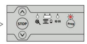
Press the button on the Keygo RTS keyfob that you want to control the Rollixo RTS controller with until the 'Prog' LED on the Rollixo RTS controller flashes and then goes out.
