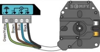
• Connect the motor wires into terminals 1, 2, 3 & 4 as illustrated above.
