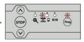
Now approach the Transmitter on the Bottom Rail – Using a small tool press the 'Prog' button on the unit until the Rollixo panel 'Prog' LED flashes, then let go (this could be up to 5 seconds) the 2 units are now active.
